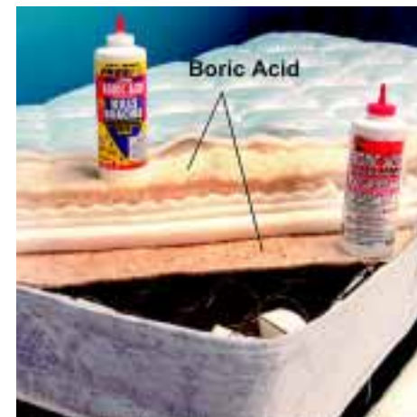
Boric Acid (Roach Killer) soaks as loose dust mixed with the cotton batting. There is 1.5 lbs of Boric Acid in the surface of a Queen mattress. Antimony Tricarbide is also included in the mixture. This is the least expensive barrier system to flameproof mattresses.
